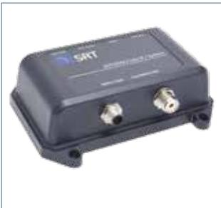
**TRANSCIVERS:** We develop advanced radio transceivers based on the international Automatic Identification System (AIS) which enables the exchange of real time data such as vessel identity, position and weather in the marine domain. Our transceiver business supplies a broad range of AIS product and module solutions which are used across a wide spectrum of applications.
